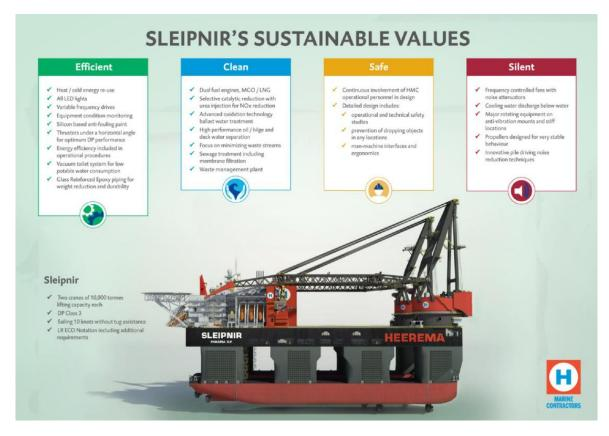
Sleipnir is the most sustainable heavy lift vessel in the world. Compared to a similar vessel using only heavy fuel oil, carbon emissions have been reduced by approximately 20%, while other emissions are reduced by at least 80%-95% and more. Sleipnir has numerous other features apart from the reduction of emissions due to the usage of LNG. Some of these are:
