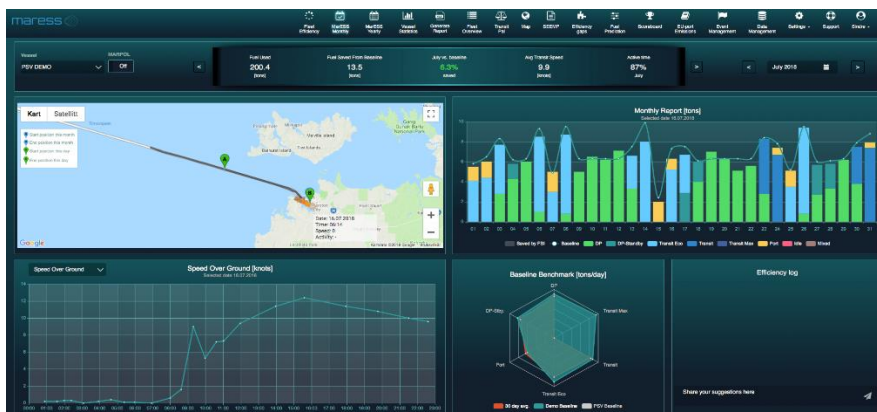
Analytics software comparing historic baseline against performance across the full range of operations of a vessel. Photo: Yxney Maritime.
