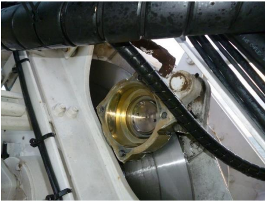
Brake housing showing sheared bolts
