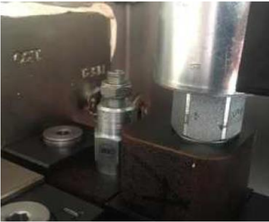
First valve with slack locking nut
