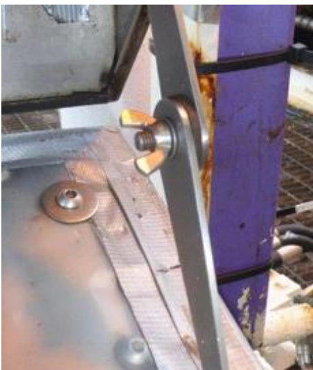
Hinged mechanism was retained by two unsecured wing nuts
