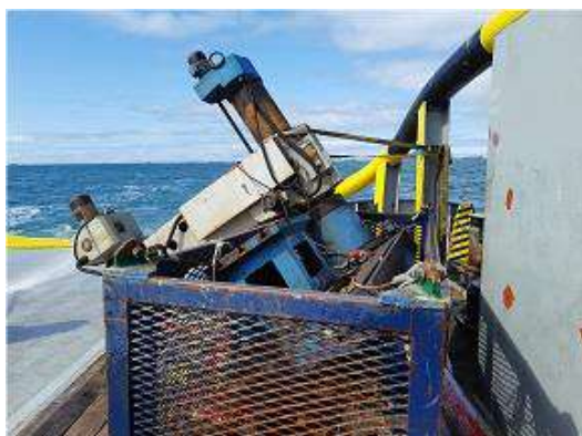
Basket with unsecured load
