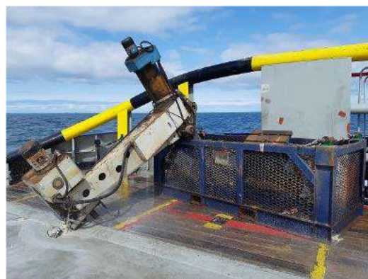
Equipment slid out of basket during lifting
