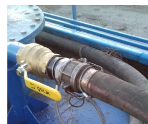
Correct connection with whip check
