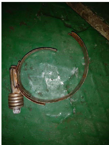
Failed hose clamp, mounted on the discharge side
