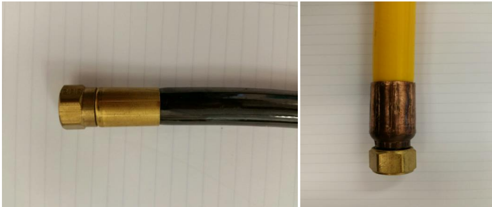
Showing crimped fittings
