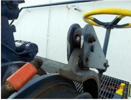
Failed section of brake assembly
