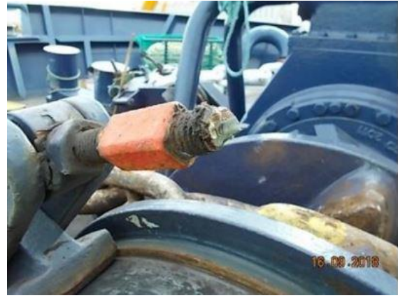
Failed section of brake assembly
