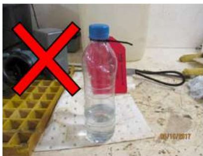
Close up of the bottle showing that the contents (Loctite SF7063) looked like water
