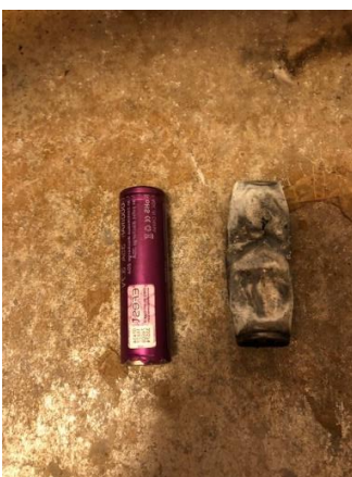
The exploded battery and the one it was supposed to replace if required.
