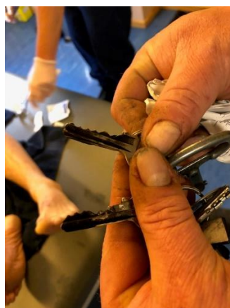
The keys that caused the short circuit
