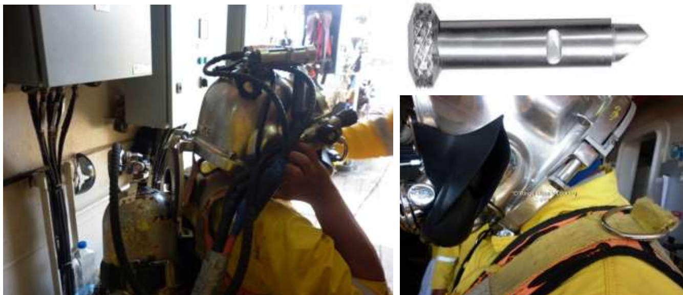
Photo indicates the open locking collar assembly in open position, behind diver's shoulders
