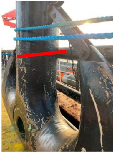
Close up of hook with intended position of rope indicated with red line
