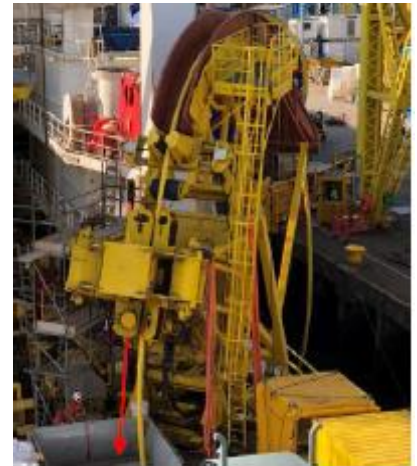
Direction of travel and landing area of tensioner pad from 20te Tri-Cat tensioner
