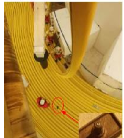
Direction of travel and landing area of tensioner pad from 20te Tri-Cat tensioner
