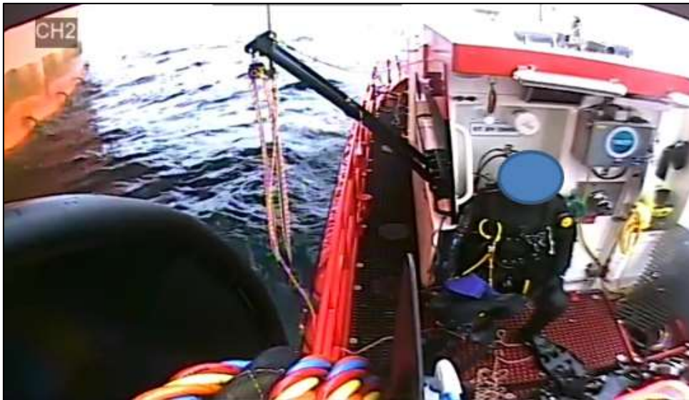
Showing mooring line caught on diver rescue davit in deployed position
