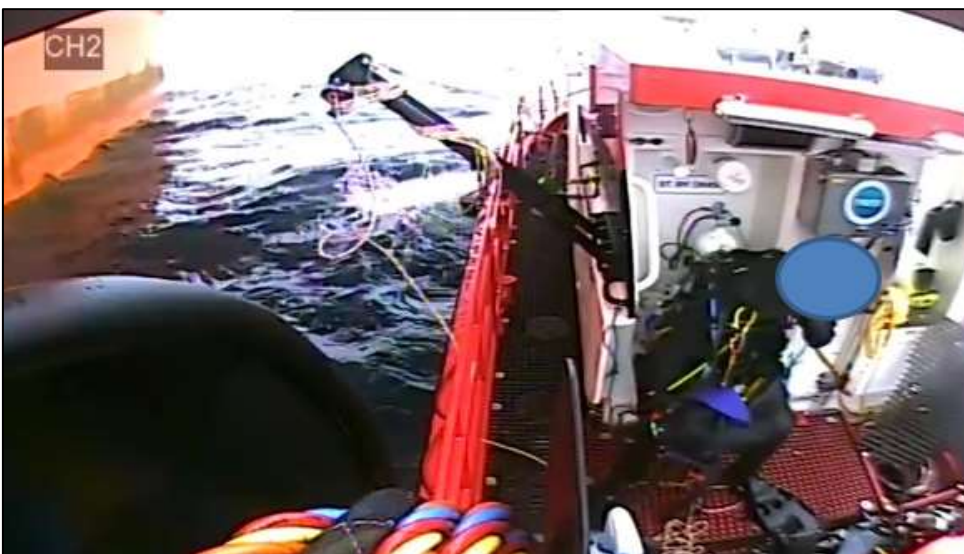
Showing block and tackle recovery device striking bulkhead
