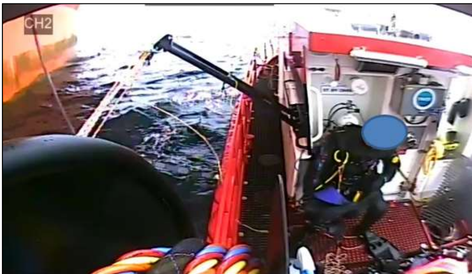
Showing tension created on the diver rescue davit by the entangled mooring line
