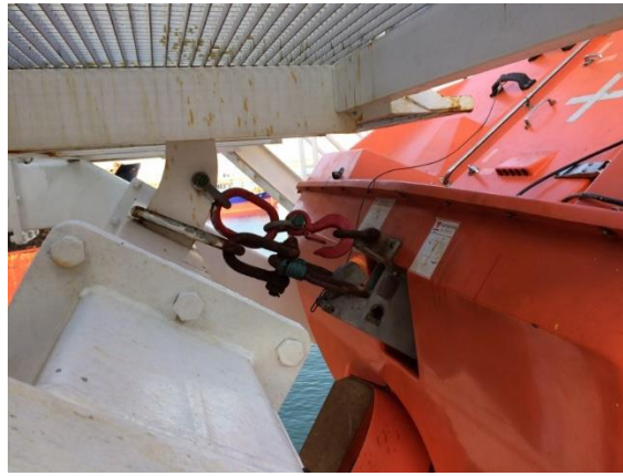
Close up of connection after retrieving back (maintenance hook applied for security)
