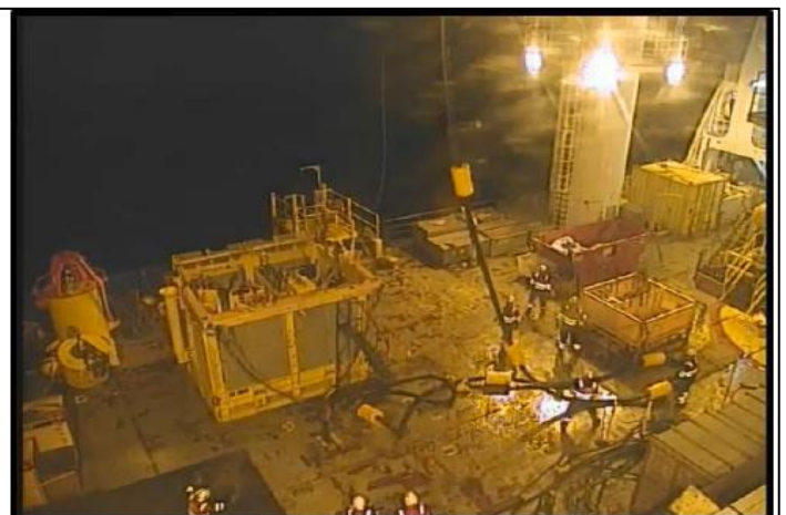
Dropped fuel hose on deck
