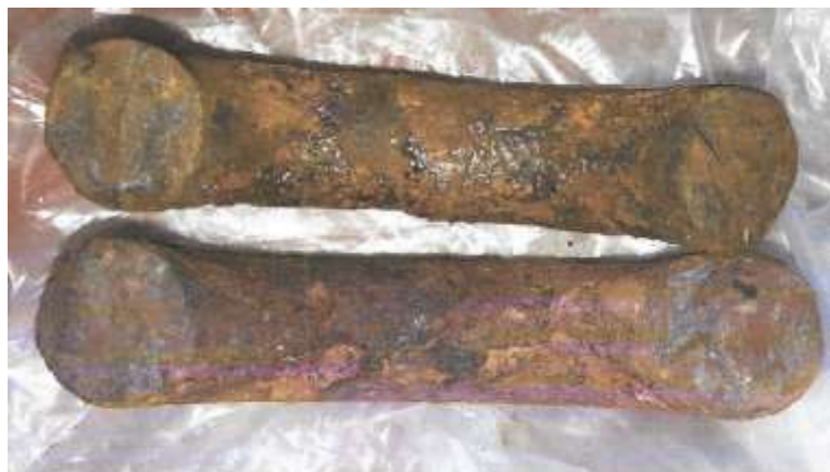
Corrosion on cross section of failure zones
