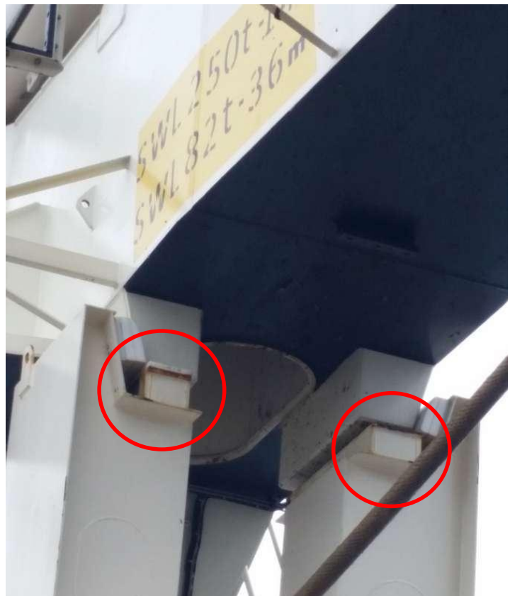
Location of Teflon pads on crane rest.
