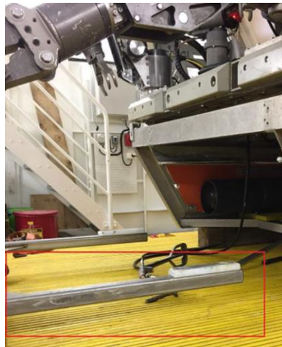
Tooling tray guide arm that made contact with the IP
