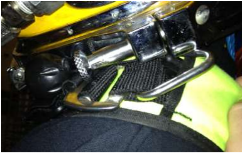
Clash between diver helmet Pull Pin and jump jacket
