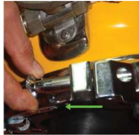
Pull Pin shown in open position
