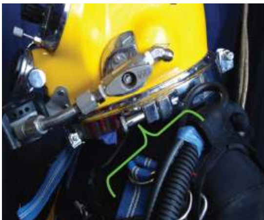
Position of Helmet/Neck Ring Pull Pins in relation to divers harness with head in normal upright position
