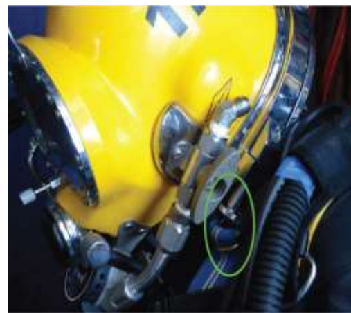
Position of Helmet/Neck Ring Pull Pins in relation to divers harness with head bent forward looking down
