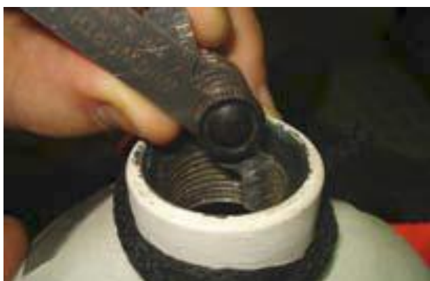
Figure: inspection of the inner thread type at a HP gas cylinder
