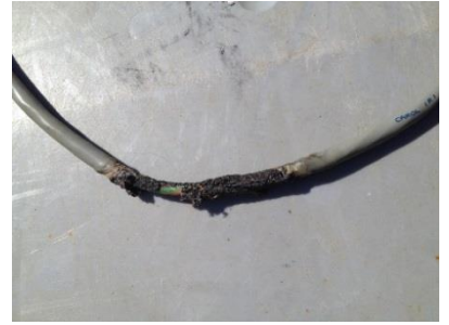
Figure: exterior sheath of the main control cable burned through;
