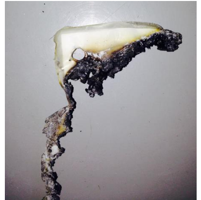
Figure: exterior sheath of the main control cable burned through;
