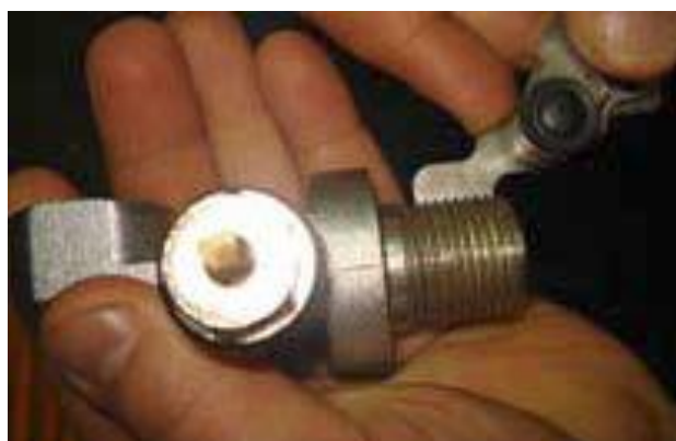
Figure: inspection of the outer thread type at a pillar valve
