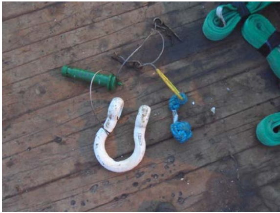
(Left): Shackle, pin and 'R-Clips' shown loose
