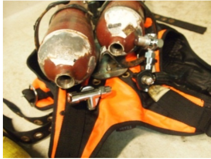
Broken manifold assembly
