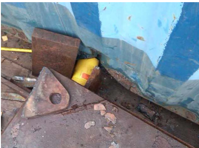
Injured person's ankle was trapped between yellow spreader bars and blue freight container
