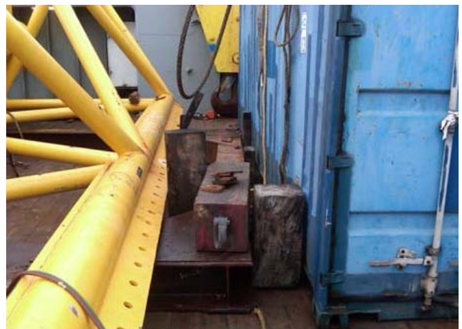
Injured person's ankle was trapped between yellow spreader bars and blue freight container
