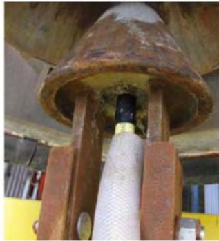
Two months after the cast was made. The strands show signs of being pulled into the cone. (Random picture available from system)
