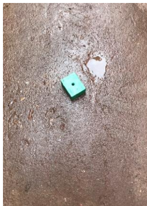
The dropped magnet – note hole for retention eyelet
