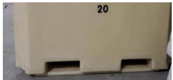
Showing correct box orientation with captive pockets presented.
