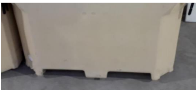
Showing incorrect box orientation with non-captive pockets presented.
