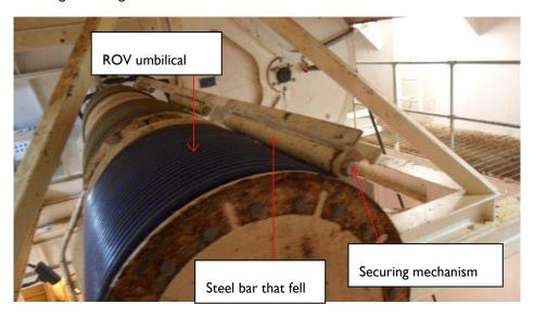
Figure: Showing ROV umbilical winch drum from which steel bar fell
