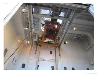
Figure: Looking to the top of the ROV hangar at the cursor and cursor winch
