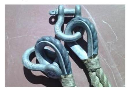
Figure: showing plastic covering under which the rope was rotten
