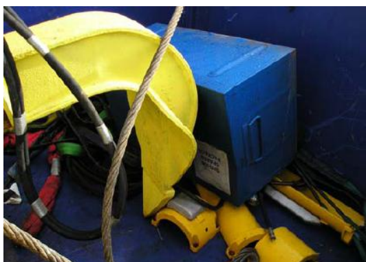
The grab handle of this blue steel case has not been secured and the case is resting on top of other equipment
