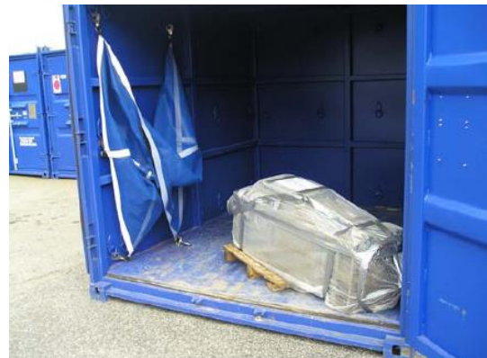
Heavy and valuable motor left unsecured for transit
