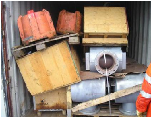
Orange clump weights (500kg) unsecured and stored on top of lighter materials
