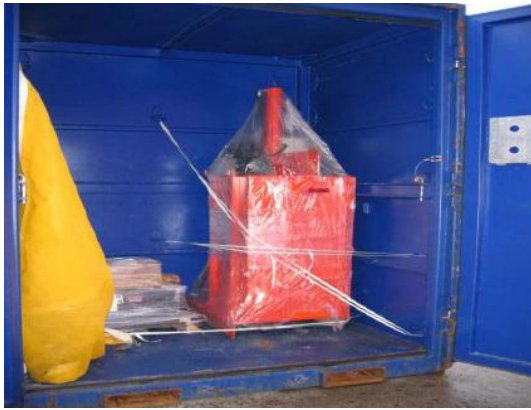
This item is secured in an inadequate manner (nylon strapping) for its weight and value
