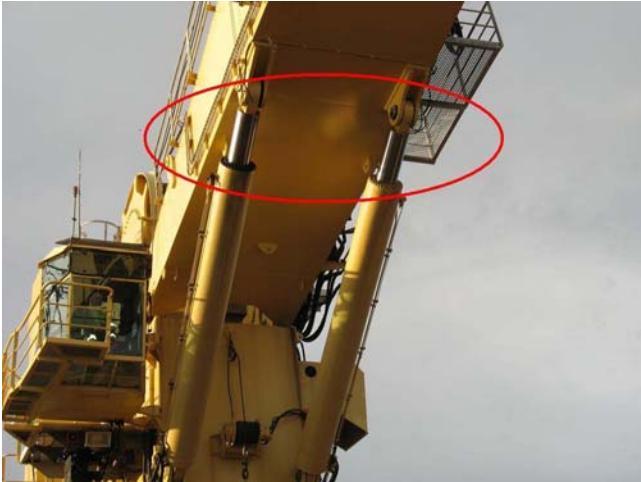
Main boom cylinders not fully closed
