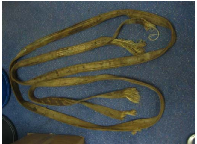
Example of worn lifting strop
