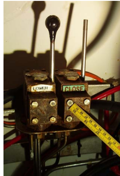
Direction control valves (DCVs) to select raiser/lower or rotate
