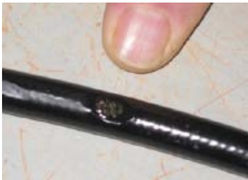
Damaged spot on hydraulic hose
