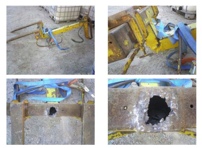
Investigation proved difficult as most of the evidence had been removed. The crate had been sent off with the garbage and the tag indicating the weight of the load was not kept. The weight of the crane motor (the load which was dropped) was established at 1.4Te, proving that the pallet lifter had failed below its SWL of 2Te.
