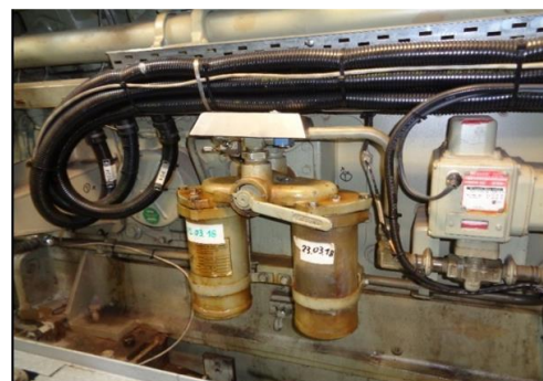
Deflector plate fitted to prevent fuel being sprayed onto the hot areas of the engine
