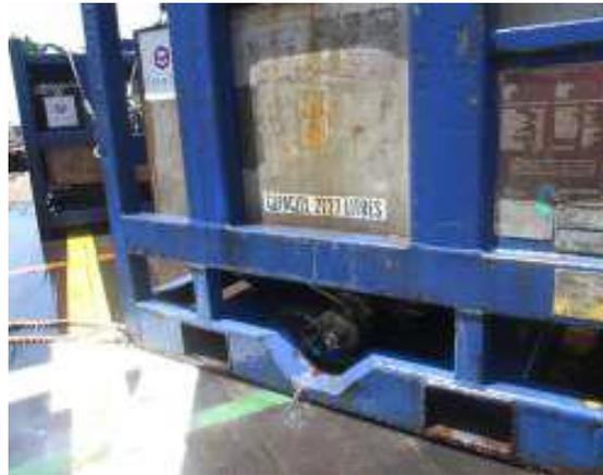
*Damaged leaking valve of the methanol tank after the incident*
