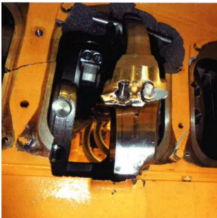
Showing the connection rod on the cylinder blown through the engine block
