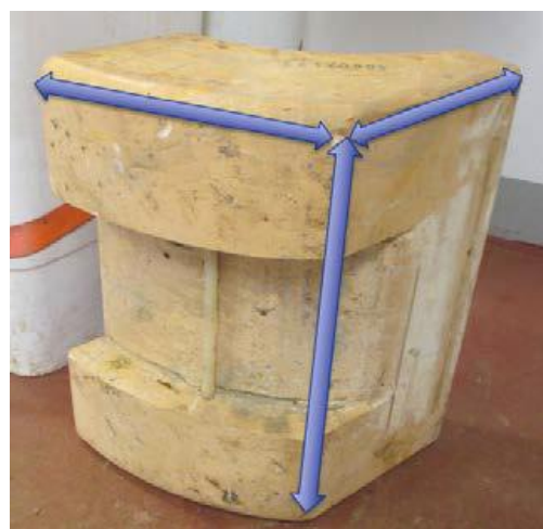
Figure 2: one of four blocks that make up inner clamp, each approx. 20cm x 25cm x 35cm and weight circa 6 kg.
