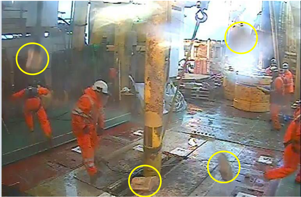
Figure 3: screen capture from a camera shows the blocks being ejected from the clamp arrangement on the riser. (yellow circles indicate the moving blocks)
