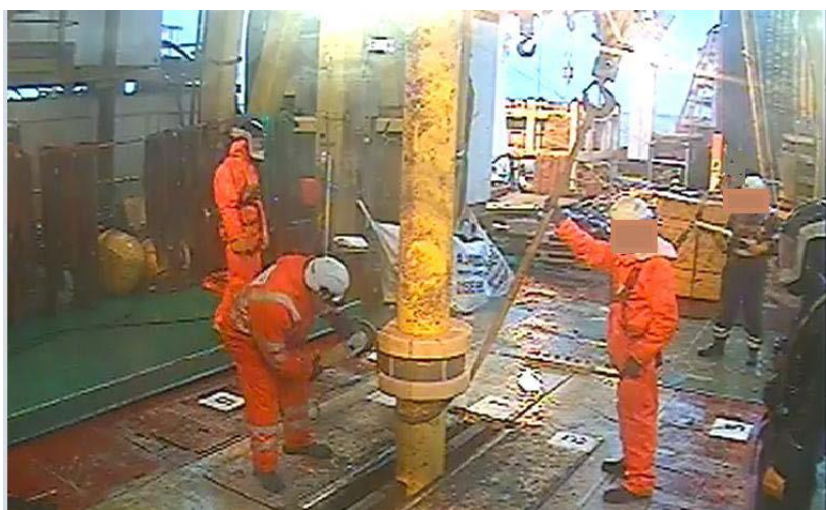
Figure 1: typical set up immediately prior to cutting band securing inner clamp
