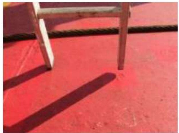
Ladder was unstable, both feet were not in firm contact with the deck
