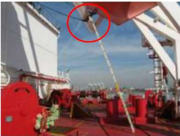
Ladder as positioned by the AB to reach the forward hook
