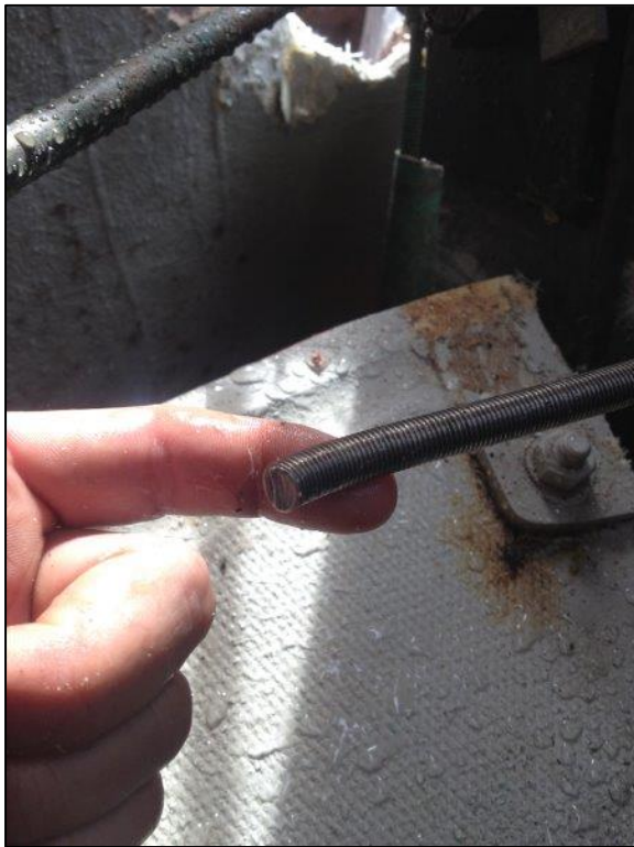
Figure 2: Showing sheared hook release mechanism from the lifeboat that dropped
