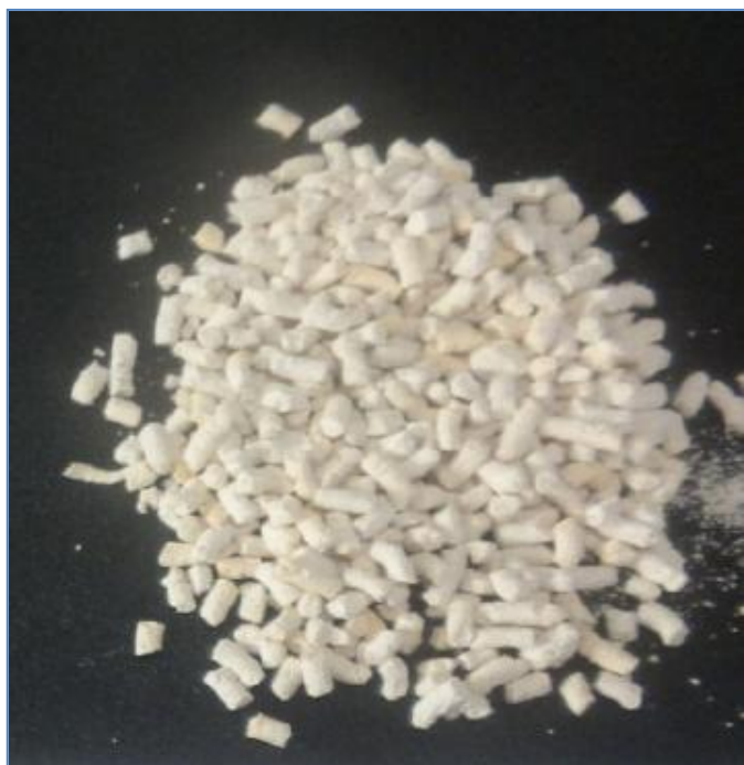
Figure: Showing the discoloured CO 2 absorbent material (note flecks of stained or off-white pellets).
