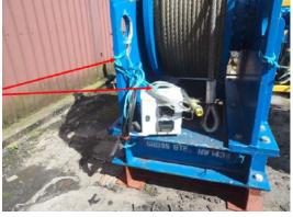
Red arrows illustrating how RLM PSU was secured to winch frame using polypropylene rope
