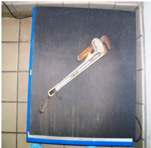
Figures: (L) pipe-wrench that fell (R) snapped single leg tether
