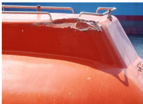
Figures showing damage to lifeboat
