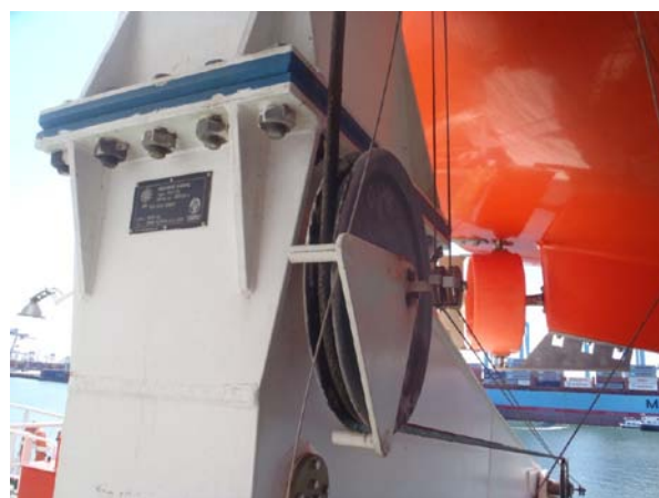
Figures showing how remote wire got stuck behind a wire sheave arrangement
