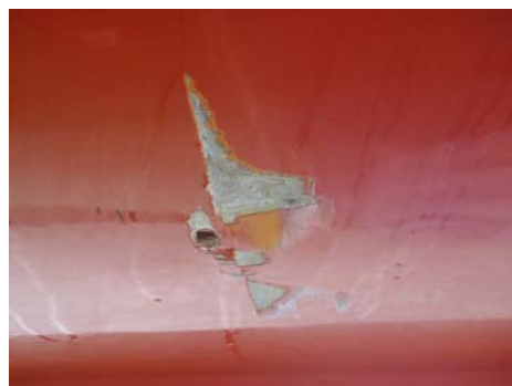
Figures showing damage to lifeboat
