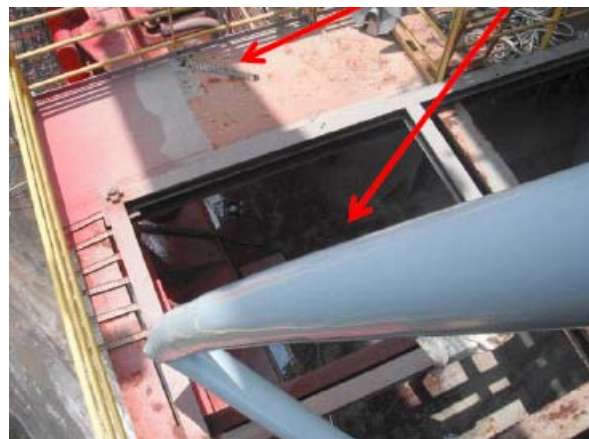
Figures: (L) Tensioner platform (R) showing where angle bar landed and bounced
