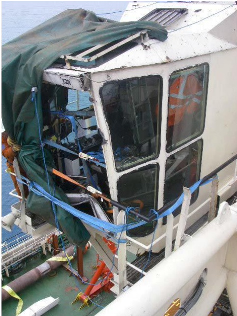
Crane cab showing damage
