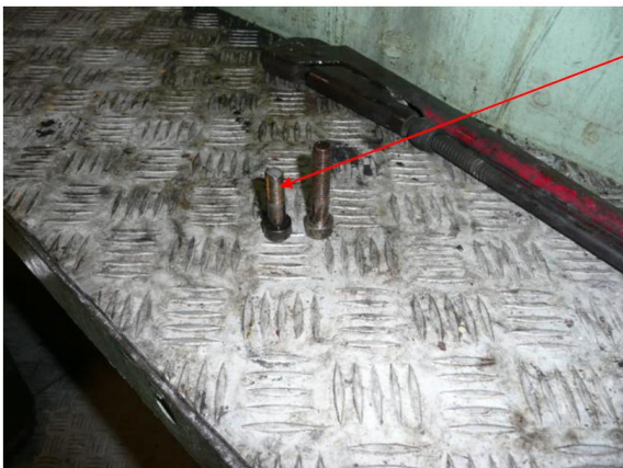
Close View of Securing Bolts that failed holding flange face of Fuel Injector Pump
