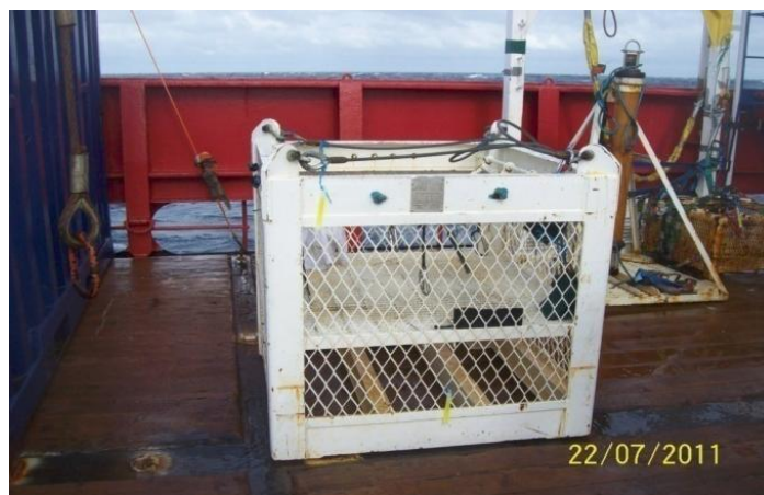
Typical 1m x 1m work basket for deployment subsea
