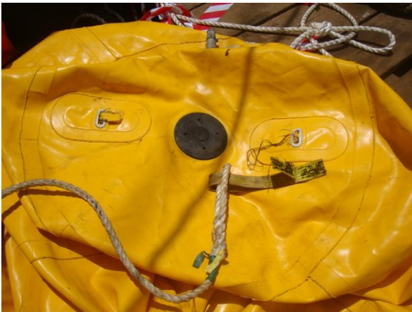
Incorrect attachment of inversion line to handling strops
