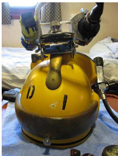
Diver's hat with the indentation where valve hit the hat
