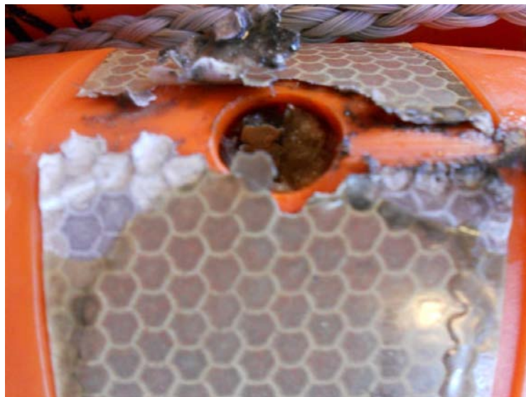
Lifebuoy Plug/stopper insert location showing lack of plug when tape removed
