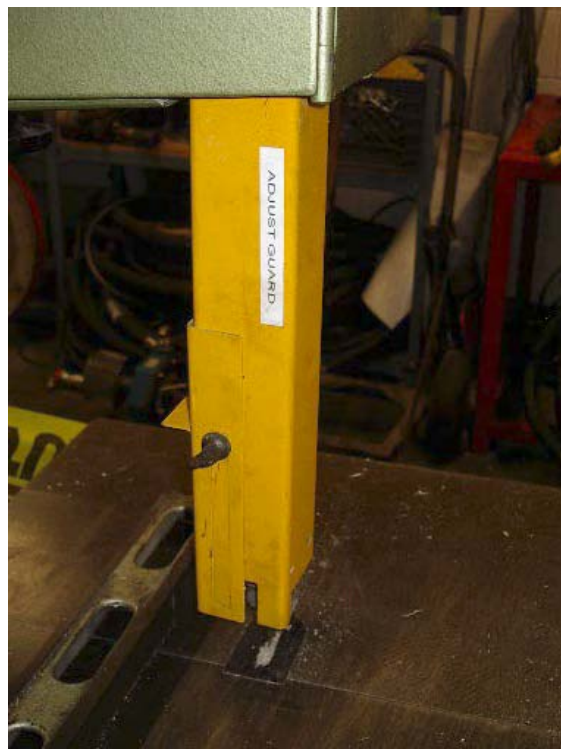
Band-saw with guard set to lowest position
