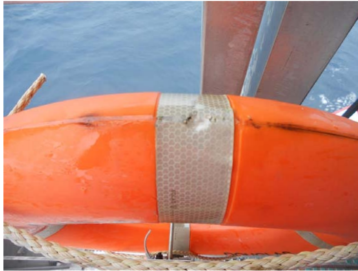
Lifebuoy Plug/stopper insert location covered by retro-reflective tape
