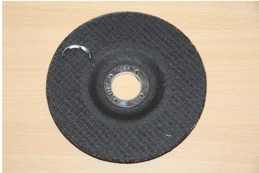
Iron ring melted into the disc
