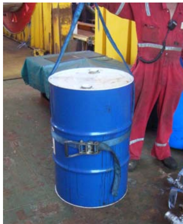
Metal drum showing intended use of barrel span set lifting strop
