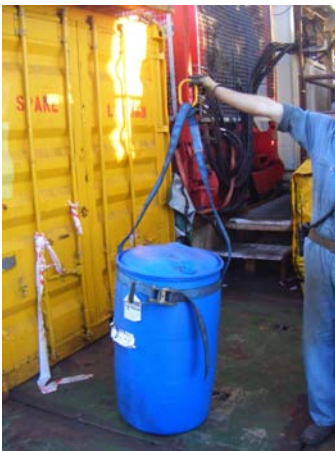
Plastic drum with curved sides with barrel span set lifting strop – poor choice as intended for metal drums
