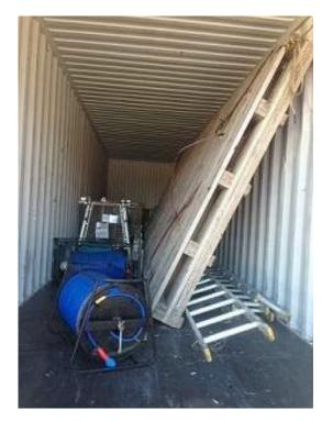
Figure: Equipment packed into a container unsecured
