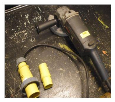
Figure: 110v/2000W/19A 9" grinder with 32amp IP67 plug and the IP44 16amp plug removed.
