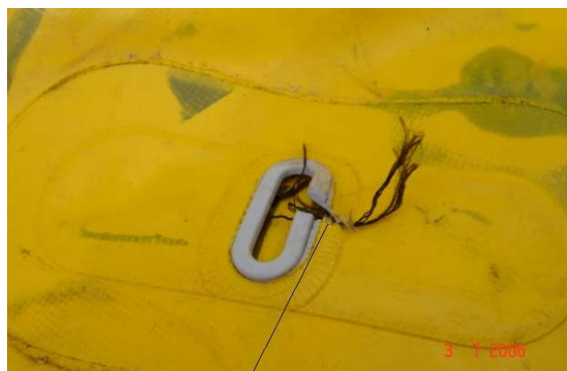
Inverter ripped out from this location
