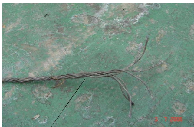
End of strop cut on flange face
