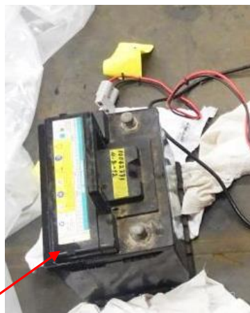
Figure: Location of vents permitting acid to leak out of battery when improperly stored
