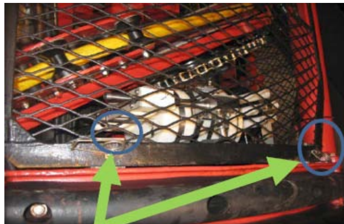
Bottom of TMS protection gate showing fixing brackets with bolts and 'R' clips which remained secured
