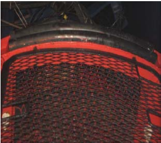
TMS protection gate showing "cut-outs" which are used as foot-holds.
