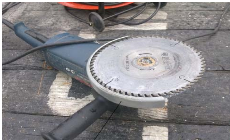
Cutting machine (with blade guard fitted)
