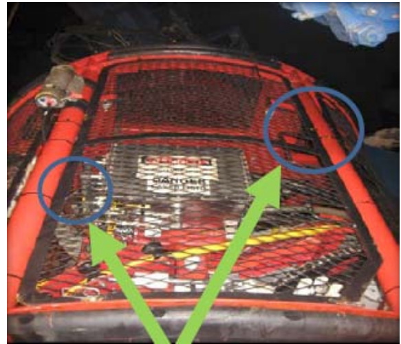
TMS protection gate showing "cut-outs" which are used as foot-holds.
