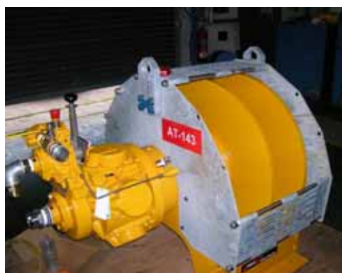
Figure 3 – Example guard for tugger winch
