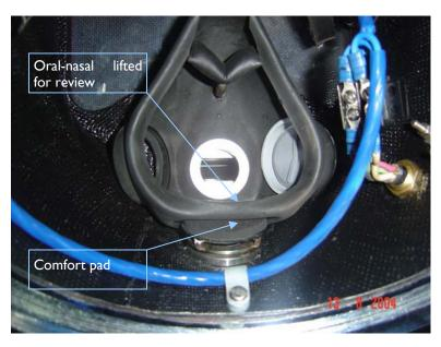
As can be seen in the photograph the part is located on top of the retaining nut at the bottom of the oral nasal piece, in close proximity to the diver's mouth. In this incident a choking incident was avoided as the part was caught in the diver's teeth during inhalation. The cause of the detachment appears to have been a loss of bonding from the adhesive which attaches the two components.
